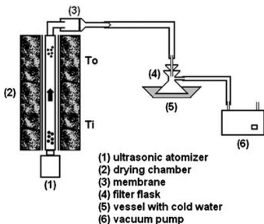
**FIGURE 3.** Scheme of the cocurrent ultrasound spray-drying system.<sup>24</sup>
